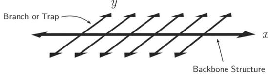
FIG. 1. Illustration of the backbone structure used in the comb model. Note that diffusion in the  $x$  direction only occurs when  $y = 0$  and diffusion in the  $y$  direction is perpendicular to the  $x$  axis.
