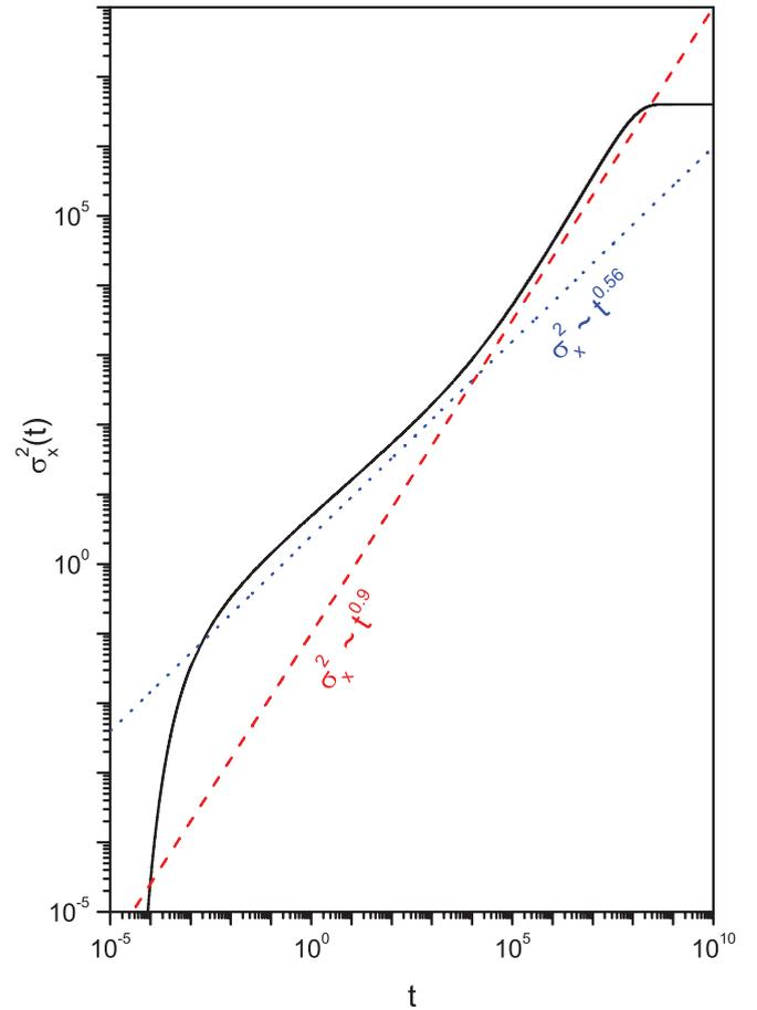
FIG. 4. (Color online) Time behavior of the mean square displacement for  $v_y = 5 \times 10^{-4}$ ,  $v_x = 0$ ,  $\bar{v}_x = 1$ ,  $\mathcal{D}_y = 5$ ,  $\mathcal{D}_x = 10$ , and  $\bar{y} = 0.1$ . The dotted (blue) and dashed (red) lines were incorporated in order to illustrate the subdiffusive behaviors presented by the system before reaching the stationary state.
