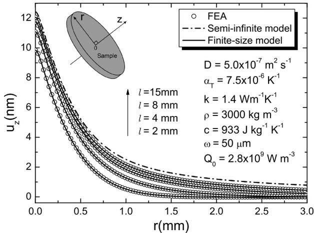
Fig. 1. Displacement profile for a standard glass [21] at  $t = 200$  ms using the finite model for different sample thicknesses (solid curves) and the FEA (open circles). Dashed curve represents the semi-infinite solution.
