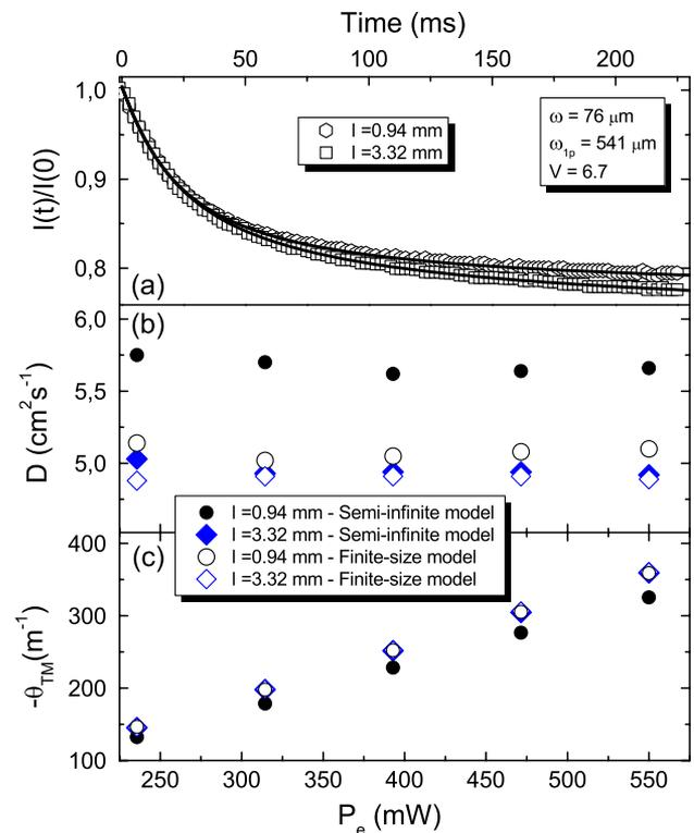
Fig. 3. (Color online) (a) Normalized TM signal,  $I(t)/I(0)$ , for glass samples;  $\lambda_p = 632.8$  nm,  $\lambda_{ex} = 488$  nm, and  $P_e = 550$  mW. Solid curves represent the theoretical fits using Eq. (10). (b) Thermal diffusivity and (c)  $\theta_{TM}$  as a function of the excitation power. The parameters were obtained fitting the experimental transients to the semi-infinite and finite models.
