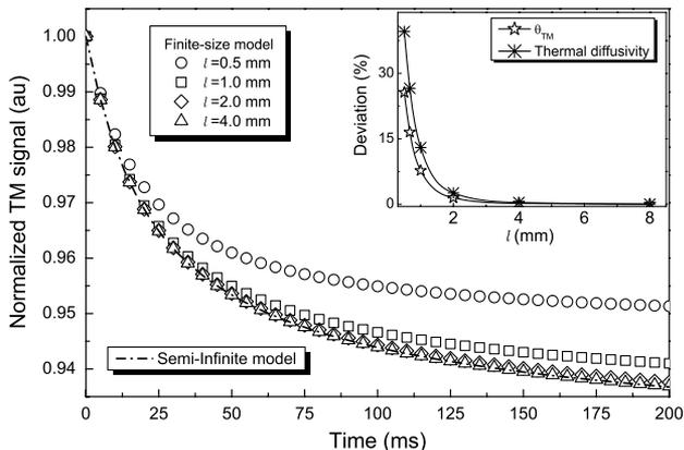
Fig. 2. Simulated TM signal for a standard glass and different thicknesses using the finite model. The inset shows the divergence between the parameters  $\theta_{TM}$  and  $D$  used to simulate the TM finite model curves and the ones obtained fitting with the semi-infinite model.
