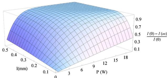
Fig. 4. (Color online) Steady-state TM signal,  $[I(0) - I(\infty)]/I(0)$ , as function of  $P_e$  and  $l$ . The parameters used in this simulation are listed in Fig. 3, and  $\theta_{\text{TM}}/P_e = 660 \text{ W}^{-1} \text{ m}^{-1}$ .
